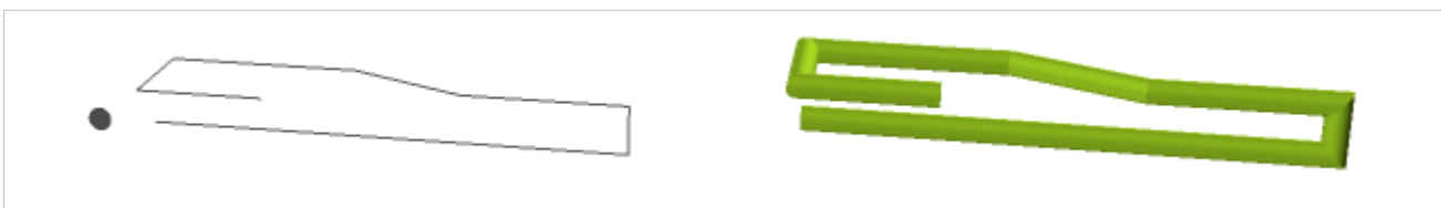
Figure 9: Extrusion of a circle along a path as possible with the Follow Me Tool.
